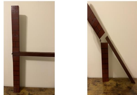
Rafters that are non fire cut may push walls out
