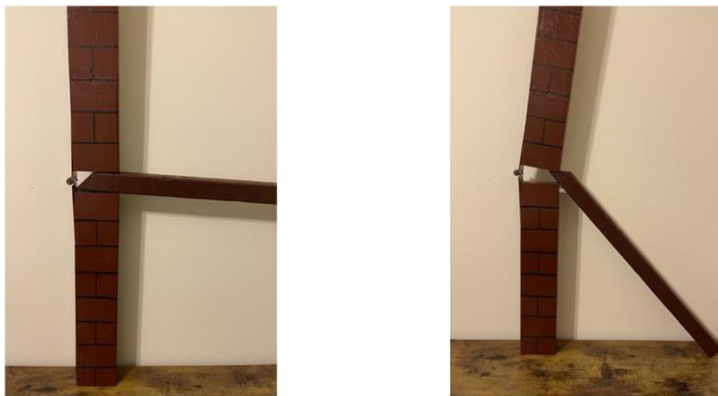
Rafters that are fire cut may cause rafters to fall inward
