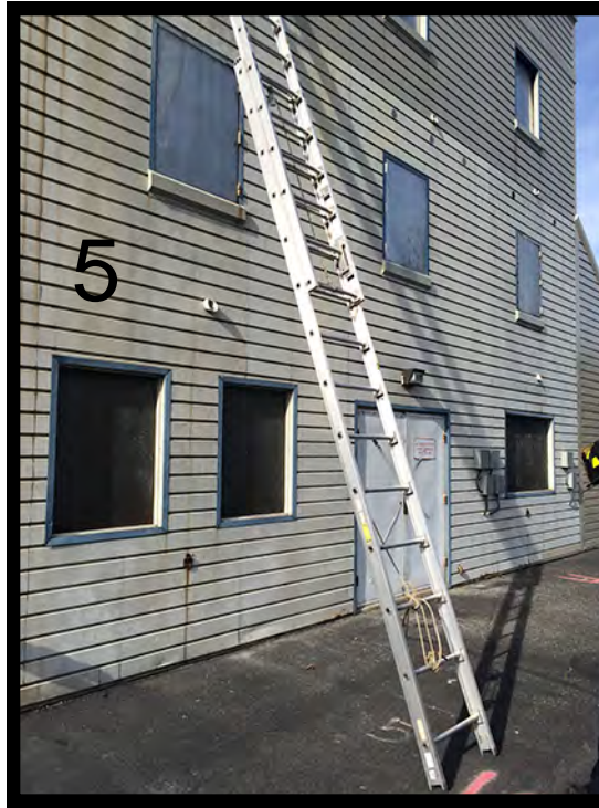
Once in place adjust if needed and tie halyard to secure ladder and communicate ladder location to units operating on the fire ground
