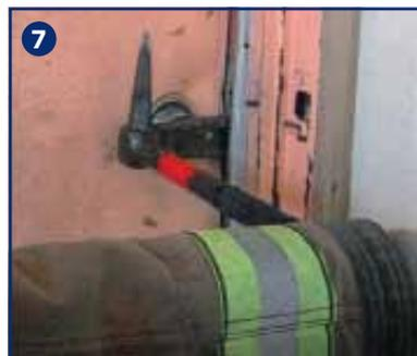
(6) A downward movement of the shaft rotates the adz. Notice that the deadbolt is beginning to fail. (7) Pulling the shaft toward the door exerts force directly on the lock.
