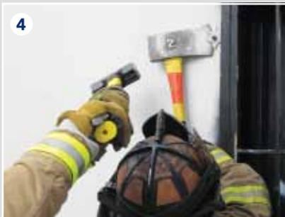
(4) An ax blade acts as a chisel and shears masonry anchor.
