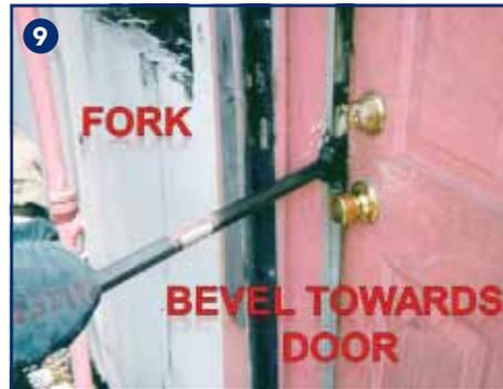
(9-10) The fork bevel is toward the door and driven deeply past the inside jamb.
