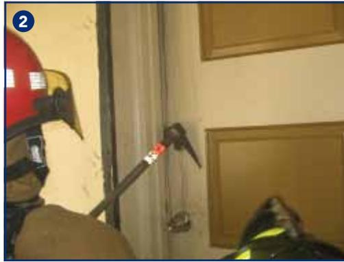
(1-2) The adz is driven into the wood doorjamb lock on the left. A downward movement of the shaft rotates the adz and forces the spike against the door. (Photos by Eric Goodman.) (3) The spike is driven into the wood doorjamb lock on the right. A downward movement of the shaft forces the adz against the door. (4) The ax blade prevents the spike from puncturing the door.
